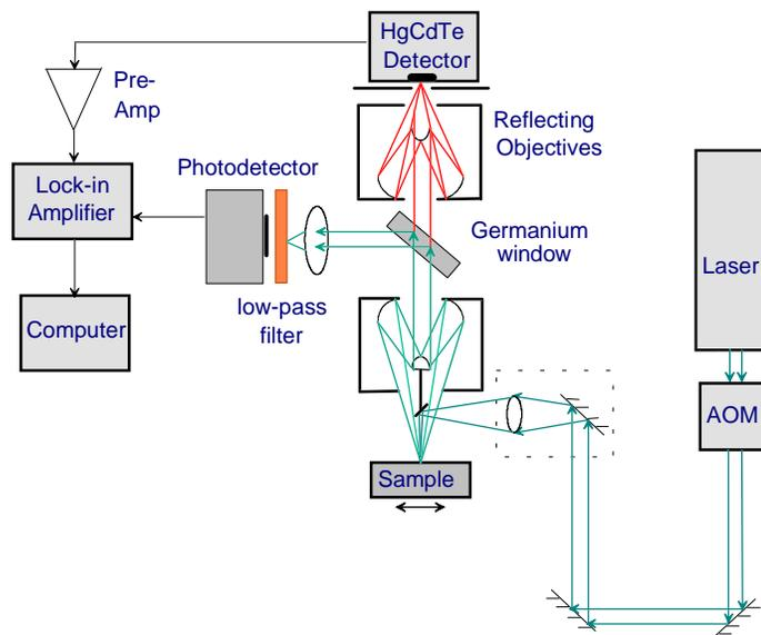
**Figure 1:** Frequency-domain photothermal radiometric (FD-PTR) and luminescence imaging instrumentation.
