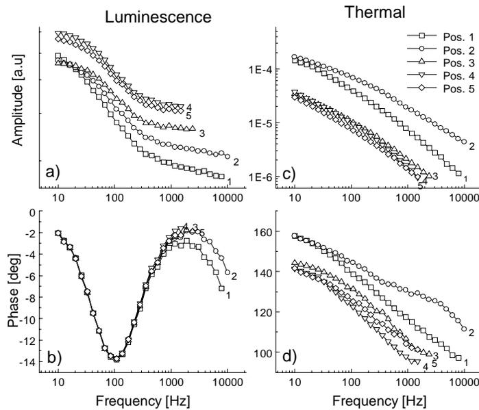
**Figure 3:** Simultaneous luminescence and FD-PTR frequency responses at five positions as shown in Figure 2. a) luminescence amplitude scan; b) luminescence phase scan; c) PTR amplitude scan; and d) PTR phase scan.
