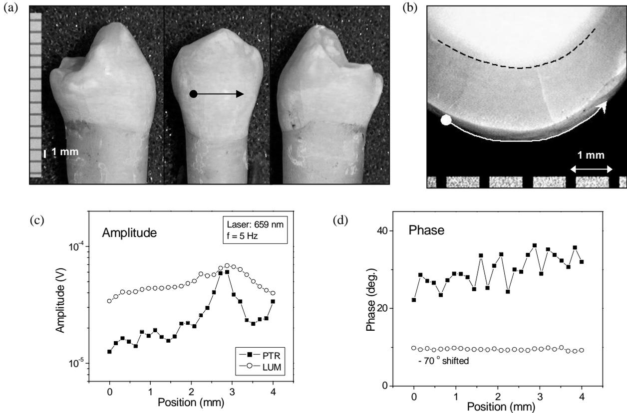
Fig. 5 Photographs and experimental results of a mandibular bicuspid with a radial enamel crack. (a) left, front, and right views of the tooth; (b) cross section at the scan level showing the radial crack. The DEJ is highlighted to aid the eye; (c,d) PTR and LUM amplitude and phase signals across the scan line at 5 Hz.
