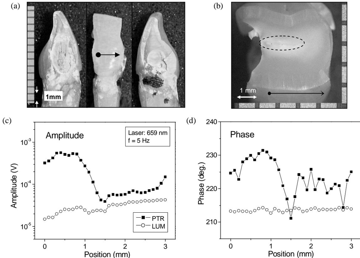
Fig. 4 Photographs and experimental results of the sample tooth having deep sub-surface carious lesion in dentin. (a) left, front, and right views of a mandibular incisor. (b) cross-section at the scan line at the level of the arrow in (a), highlighting a deep demineralized lesion (dotted region in the middle); (c,d) PTR and LUM amplitude and phase signals across the scan line at 5 Hz and 659 nm.
